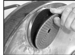
When setting machine down into operation position, hold machine firmly. Set down gently, DO NOT drop. Damage to accessories and machine could occur if dropped.
